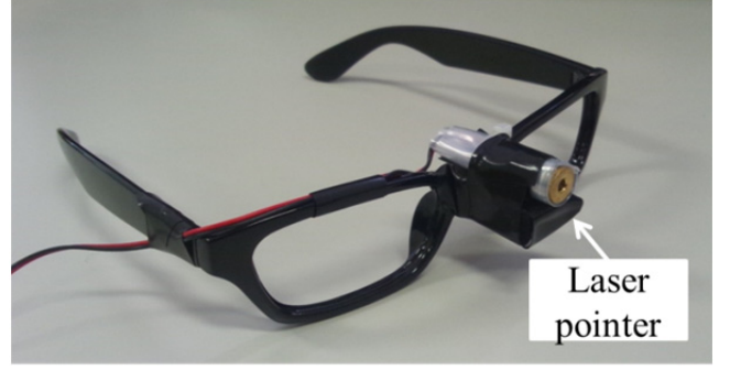
Fig. 8. A conventional pointing device (eyeglasses equipped with a laser pointer)
