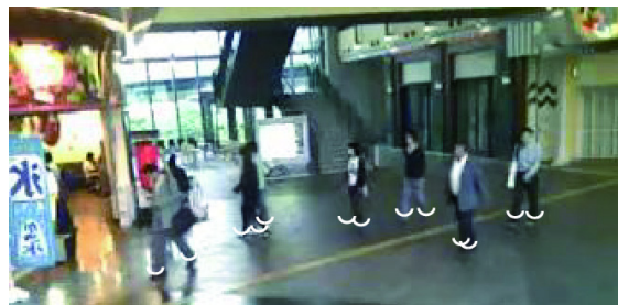
Figure 2: Pedestrian walking in a shopping mall. The white marks represent the detected legs of pedestrians. Walking rhythm of each pedestrian is observed using wearable accelerometer and LRFs by tracking at least one foot.
