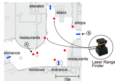
a) Positions of LRFs (shown as red circles) in the experimental environment.
